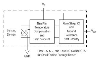
Figure 1. Fully Integrated Pressure Sensor Schematic
