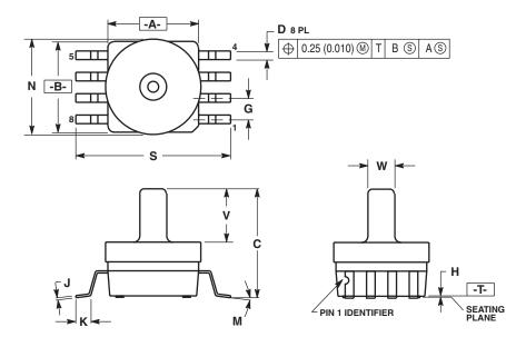
NOTES: 1. DIMENSIONING AND TOLERANCING PER ANSI Y14.5M, 1982. 2. CONTROLLING DIMENSION: INCH. 3. DIMENSION A AND B DO NOT INCLUDE MOLD PROTRUSION. 4. MAXIMUM MOLD PROTRUSION 0.15 (0.006). 5. ALL VERTICAL SURFACES 5' TYPICAL DRAFT.
