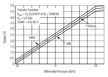
Figure 2. Output versus Pressure Differential
